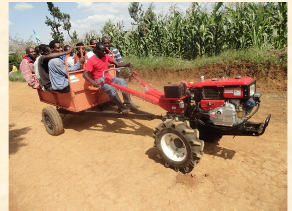
Power tiller yambaye remoroki itwara toni y'umusaruro.
