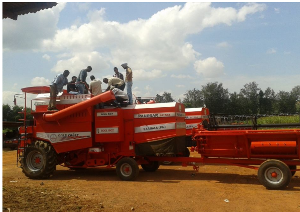
Imashine isarura umuceri, ibishyimbo, ibigori n'ibindi yitwa Combine Harvester
