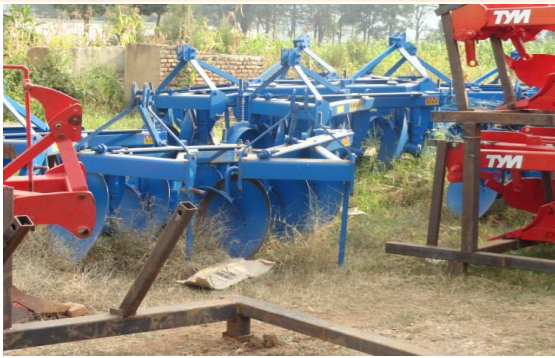
Amsuka akoreshwa n'imashini z'amapine ane (tractor) zihinga ahantu hakomeye (Disk Plow).
