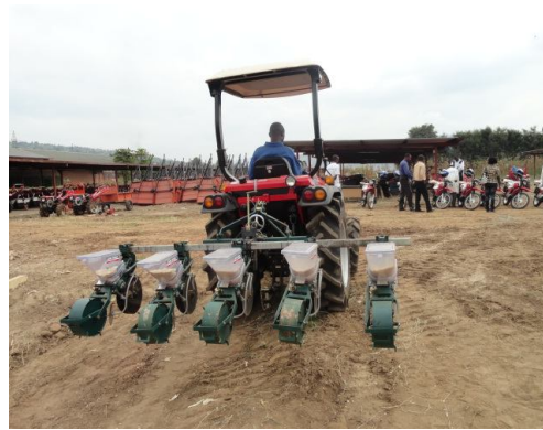
Imashini ikoreshwa mu buhinzi ifite amapine ane (tractor) yambaye amasuka yayo yo gutera ibinyampeke bitandukanye.
